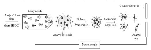
Figure.4.Adapted schematic of electrospray ionisation
