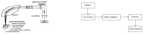
Figure.2.Schematics of a simple mass spectrometer with sector type mass analyzer
