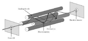
Figure.6.Schematic of the Triple Quadrupole Mass Spectrometer
