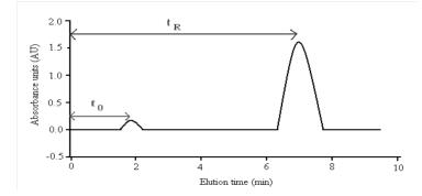
Figure.1.Schematic of a typical HPLC chromatogram
